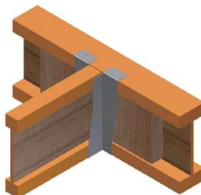
Figure B4 – Enhanced top fix I-joist to I-joist.
