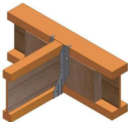
Figure B1 – Standard face fix I-joist to I-joist.
