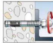
5: Turn on the washer and Upat MAX dome nut
